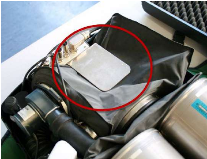
Fig. 48 Blocking surplus valve on exhalation bag
