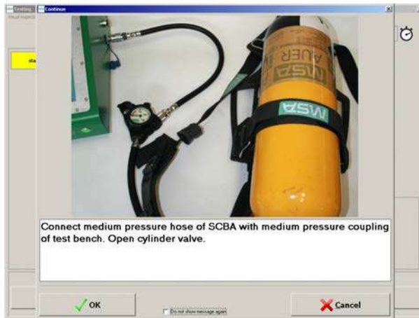
Fig. 37 Connecting the compressed air breathing apparatus
