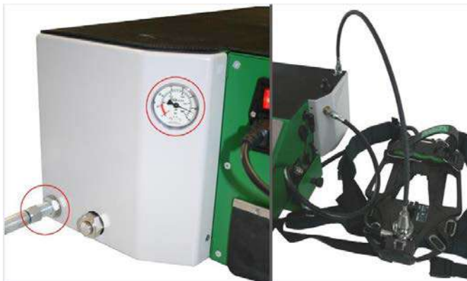
Fig. 36 Connecting high pressure line
