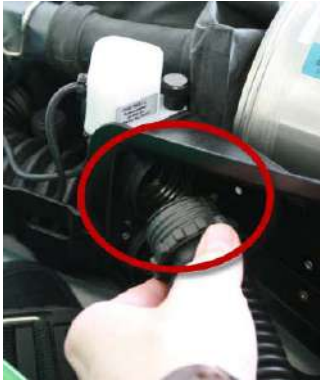
Fig. 45 Screwing adapter into inhalation side
