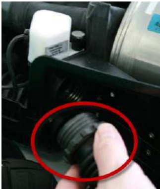
Fig. 46 Screwing adapter into exhalation side
