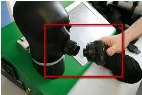
Fig. 47 Connecting breathing hose assembly to test head
