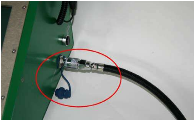
Fig. 31 Connecting medium pressure line
