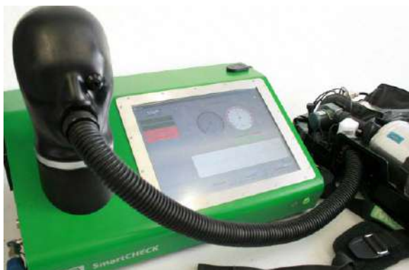
Fig. 44 Connecting adapter hose to test head.
