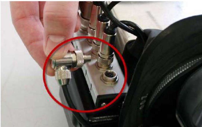
Fig. 43 Disconnecting battery of closed circuit breathing apparatus
