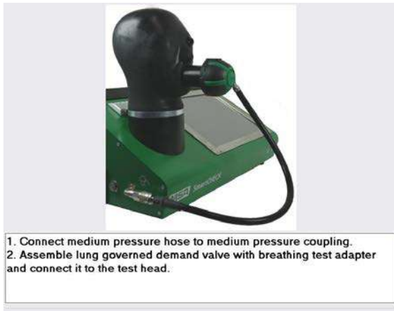
Fig. 34 Connecting the lung governed demand valve
