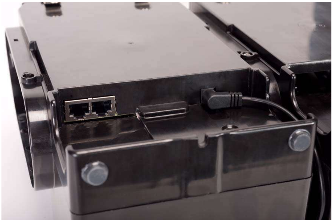
Fig. 6 Test Stand Ethernet jacks
