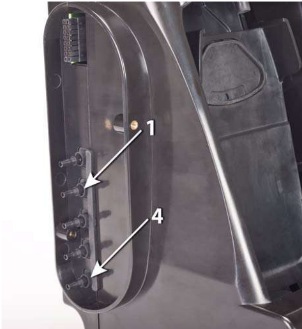
Fig. 17 Gas inlets on the Test Stand
