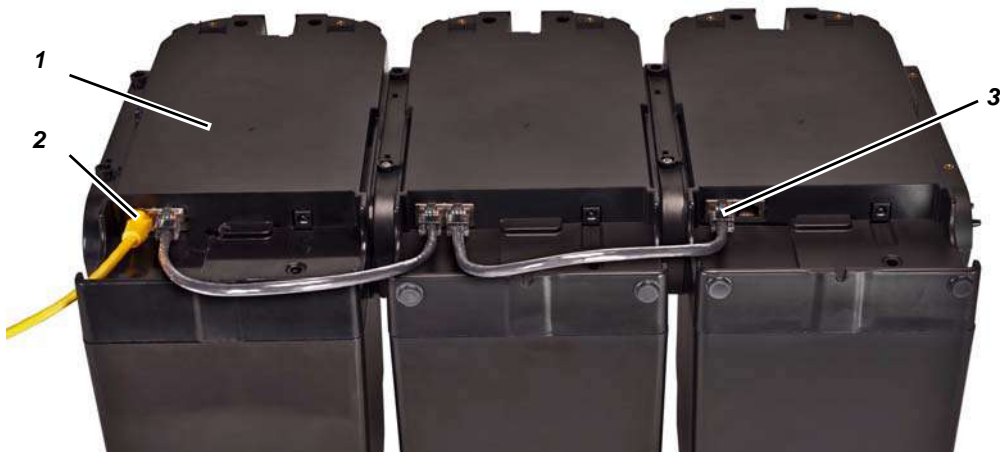
Fig. 11 Test Stand Ethernet connections
