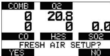
Fig. 6 Fresh Air Setup
