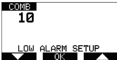
Fig. 8 Sensor Alarm Setup
