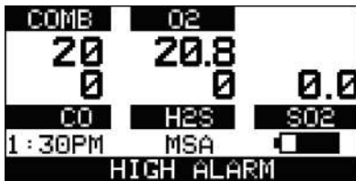
Fig. 5 Alarm Conditions (here High Alarm)
