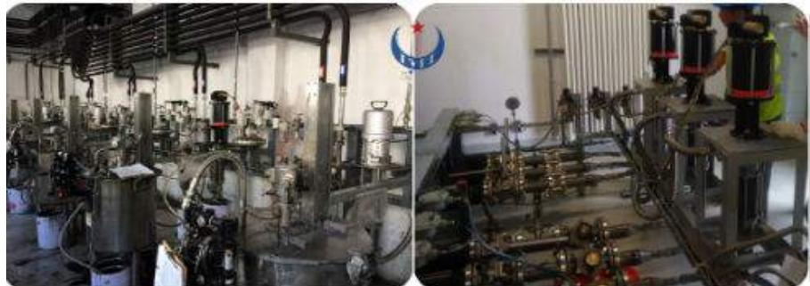
Bơm sơn tuần hoàn/Circulating paint pump
