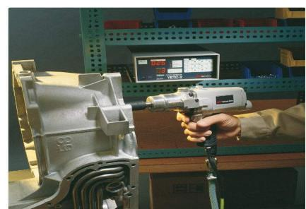
Combine the power and ergonomics of reactionless pulse tools with closed-loop electronic control to maximize productivity in torque-critical applications.
