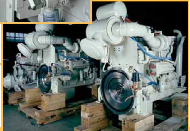
IR's genuine 150BMGE21RH-6R remanufactured starter is shown mounted on a Detroit Diesel 12V-71R.
