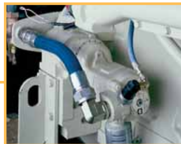
The 150BMGE21RH-6 starters are shown mounted on a Cummins KTA14-M3 and KTA19-M4I.
