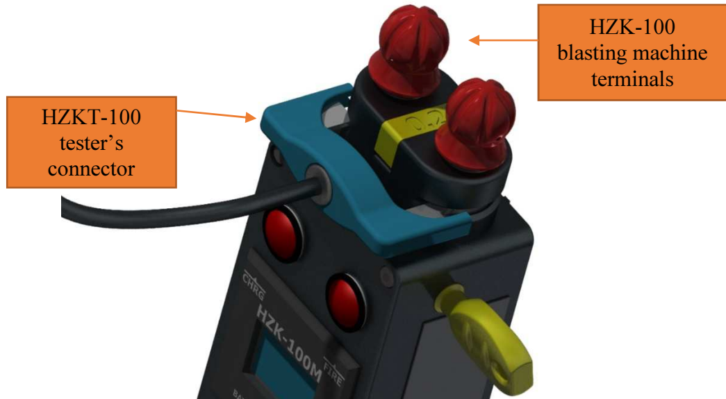
Figure 8.1 Connection of HZKT-100 tester to HZK-100 blasting machine
