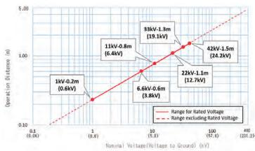
Operation Voltage-distance table and graph are theoretical value. Operation distance is varied depending on the actual surrounding environment. Please confirm operation distance in actual use environment before using.
