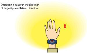
In the direction of the palm, the detecting distance is shorter than in the upper direction.
