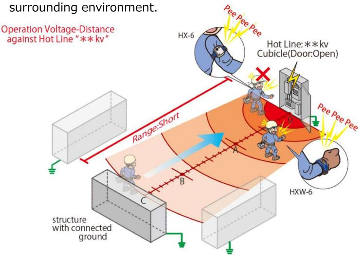
Operation Voltage-Distance Table and graph are theoretical value. Please confirm operation distance in actual use environment before using.
