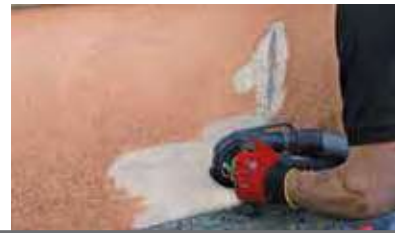
PCD milling disc for concrete surfaces (P/N 37125000)
