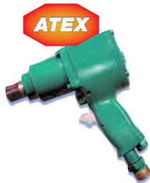
6 1316 0050 3/4" Pneumatic Impact Wrench 995 ft-lbs. torque
