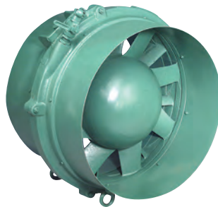
8 1524 0300 Pneumatic Axial Fan, 24" dia. 12,353 cfm output @ 90 psi
